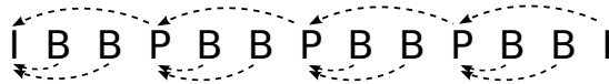
Fig. 3 Concealment algorithms te_2 and te_3 : reference frames used in case of loss for a typical GOP pattern.
