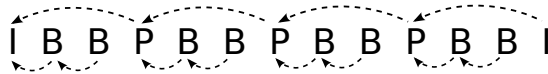
Fig. 2 Concealment algorithm te_1 : reference frames used in case of loss for a typical GOP pattern.
