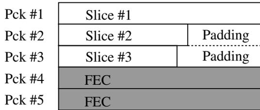
Figure 2: Cross-packet redundancy (padding scheme).
