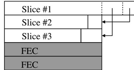
Figure 3: Packet size equalization scheme with slice splitting.
