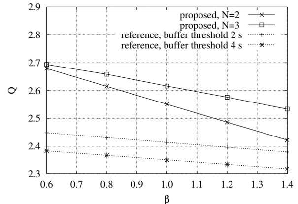
**Fig. 3.** Comparison of the proposed technique and the one in [4] in terms of video quality as a function of the  $\beta$  parameter. Average over all the traces.
