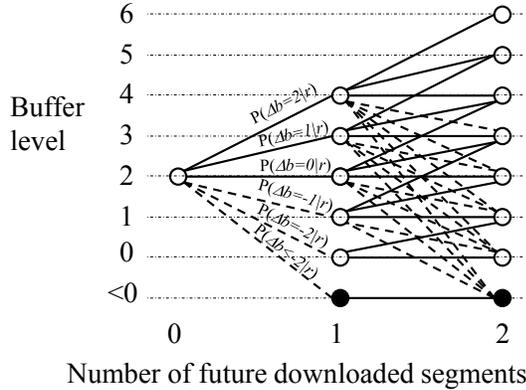
**Fig. 1.** The trellis representing the possible situations of buffer level once a given number of segments have been downloaded (2 in the figure). The size of the segment is assumed to be 2 frames. For all dashed edges the download rate is lower than the rate of the requested representation  $r$ . The objective is to compute the probability of the black-filled nodes representing a freeze event.
