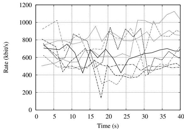
**Fig. 2.** The rate of the eight HTTP download speed traces used in the experiments as a function of time.
