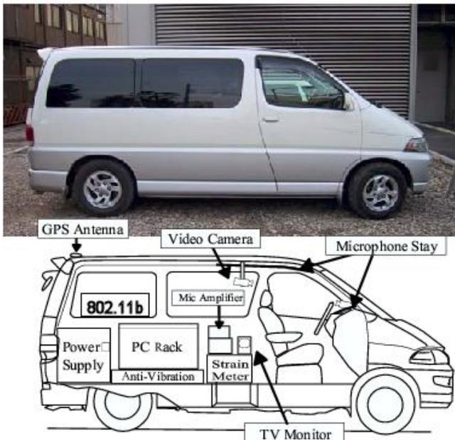
Fig. 1. Data collection vehicle used during the experiment.
