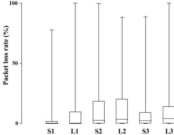
Fig. 4. Raw packet loss rate data for urban scenario presented with box-plots. The line in the middle of the box indicates the median value, the upper and lower bounds of the box indicate the third and first quartile respectively ( $Q_3$  and  $Q_1$ ) and the external lines extend until the adjacent values.
